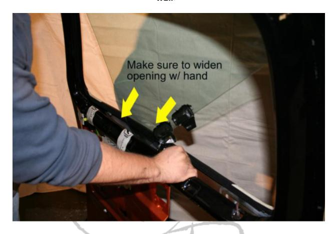
IMPORTANT STEP: Install the new 10mm nuts on the brackets and then roll the window all the way up.
