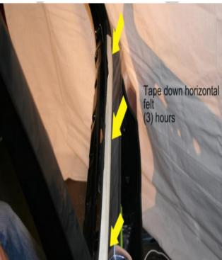
Make sure not to over-glue the new scraper and tape down after it has been lined up between both ends. The Tape can be removed after about 3 hours.
