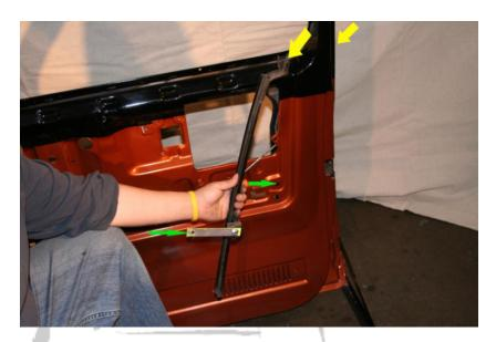
After you remove the rear vertical guide, find the 4" extension that is included in your kit and bolt one end of it as seen in the picture below. The hole on the opposite side is for the original hole on the door skin which will push the guide closer to the door latch assembly
