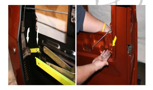
• Don't Forget to Slot the Hole for future adjustment
