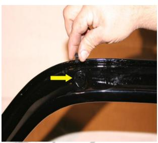
**#13.** In step we will be installing **the felts**, including **the inner and outer scrapers** and **the required backspacer**. **Quick Tip**:
