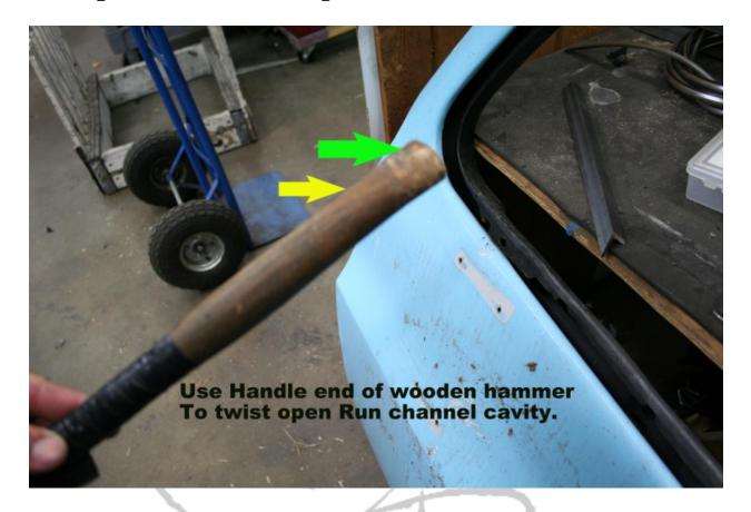
Use Wooden end of a hammer to twist open the cavity of the New Run Channel. Open to roughly about 1" wide measured from the inside.
