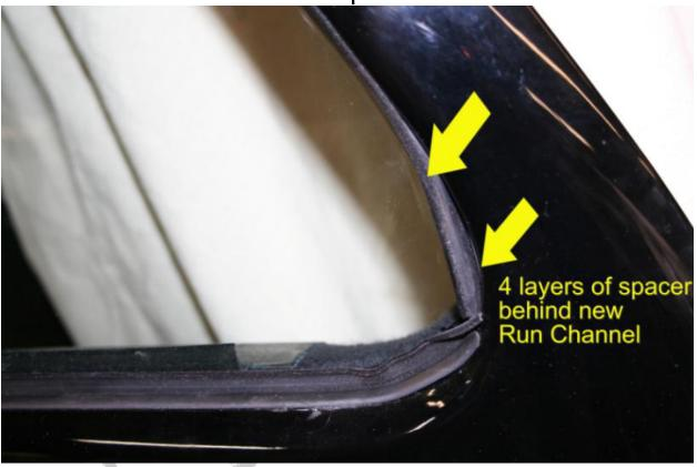
\*\*\*Tip to remember: Some trucks will only require 3 layered spacers while others will require the full four. I like to also use expanding insulation foam that is used on houses. You can pick this up at any Home Depot.\*\*
