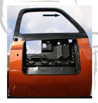
**#5.** After the Door Glass and Vent Glass Assembly have been removed, continue to remove all the old felts and scrapers (the old brittle fuzzy stuff) that are left on the door.
