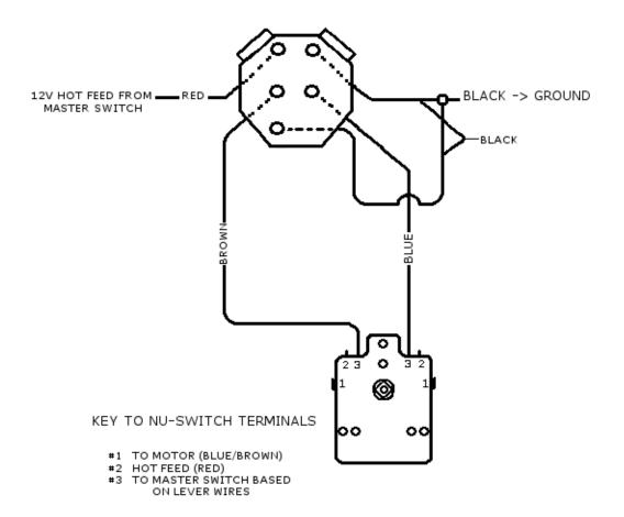
Wiring Instructions for a Singe Master Switch for Nu-Cranks
